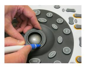
3. Moisten a cloth with rubbing alcohol or warm water. (\*Make sure it is mildly damp and not dripping with liquid). Clean the trackball itself then clean the clear plastics underneath thoroughly. Use a dry cloth to remove excess liquid and verify it is completely dry prior to reassembling.
