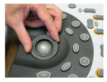
5. Secure the retainer ring into place by inserting the pen in the left indentation and pushing towards the back of the computer to spin the ring clockwise. It should lock back into place when the dots become parallel with the computer bezel.
