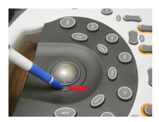
2. The ring will disengage and start to lift. Gently remove the ring then remove the ball.
